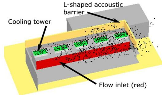
**Fig. 16.** Close-up snapshot, using SmokeView, of water-vapor particles emanating from the cooling towers and re-entraining into the flow inlet (shown in red). (For interpretation of the references to color in this figure legend, the reader is referred to the web version of this article.)
