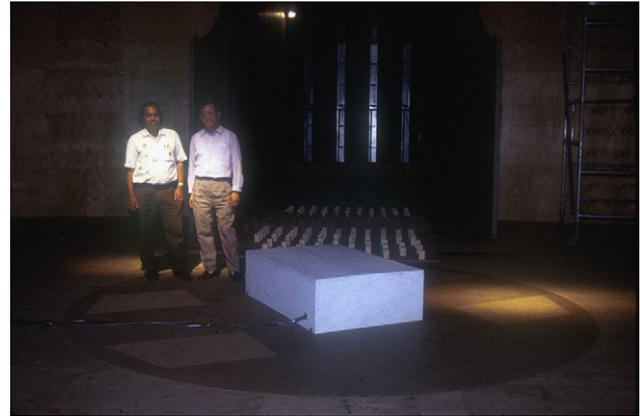
Fig. 6. 1:10 TTU Building model in the large Monash University wind tunnel (after John Holmes).
