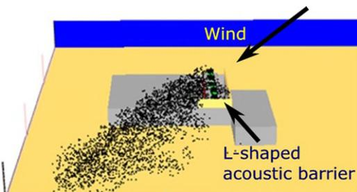
**Fig. 15.** An instantaneous snapshot, using SmokeView, of particles depicting the transport and dispersion of the cooling tower water-vapor plume. Note direction of wind and location of acoustic fence.
