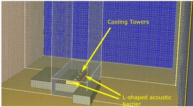
**Fig. 14.** Computational grid to study re-entrainment of cooling tower plumes into flow inlets due to addition of an acoustic barrier surrounding the towers on the edge of the building roof. Grid resolution is refined in the vicinity of the acoustic barrier and cooling towers (white-line box) to capture the flow physics more accurately.
