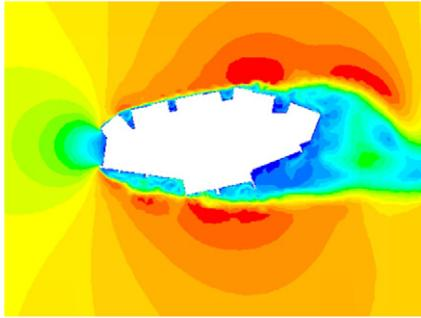
**Fig. 10.** The flow is from left to right in this LES, unsteady, snapshot of the velocity magnitude contours (blue=0 m/s and red=15 m/s). This initial design formed a baseline for modifying the building shape to reduce the crosswind response (after CPP Inc.). The full flow video may be seen at [www.aawe.org](http://www.aawe.org). (For interpretation of the references to color in this figure legend, the reader is referred to the web version of this article.)
