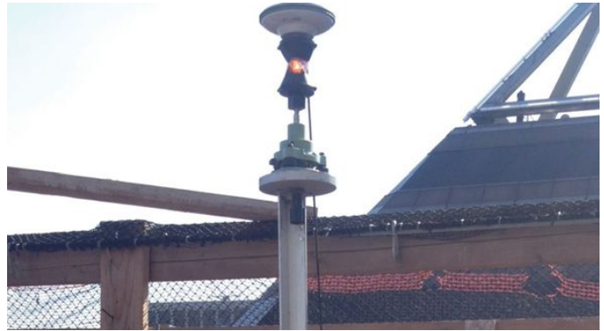
Continuously monitored optical data, derived from total station shots on 360-degree prisms mounted just beneath the GNSS receivers, give feedback on the building's frame and shape. Prisms also are used as resection points when doing layout and form positioning work.
