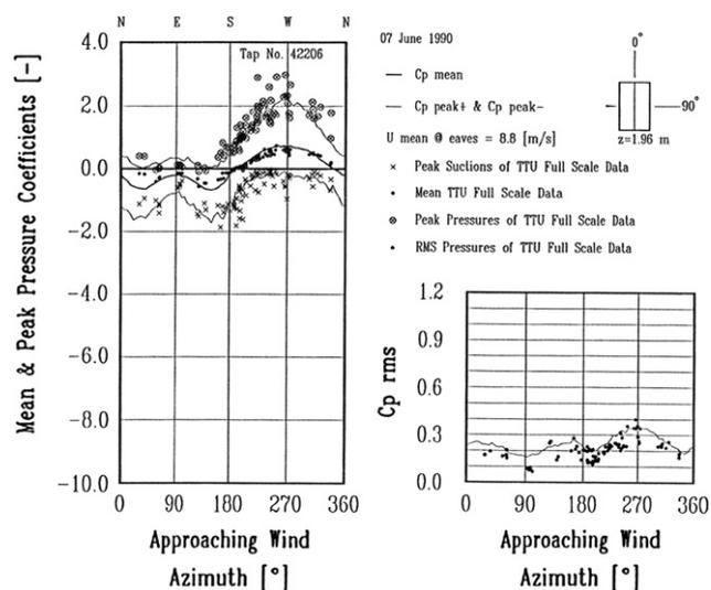
Fig. 3. Full-scale and model-scale (1:100) pressure coefficient data for the Texas Tech Building for a tap located at the center of the long wall (after Cochran, 1992).
