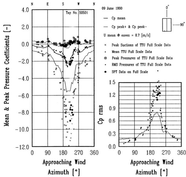
Fig. 4. Quartering winds at the roof corners produce roof-corner vortices. Wind-tunnel data do not capture the same magnitude of peak coefficients due to the relative tap size (see SPT data) and Reynolds number influences discussed below (after Cochran, 1992).
