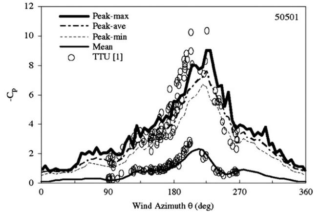
**Fig. 8.** Range of peak pressure coefficients from a model of the TTU Building collected by multiple ergodic experiments in the wind tunnel (after Endo et al., 2006).
