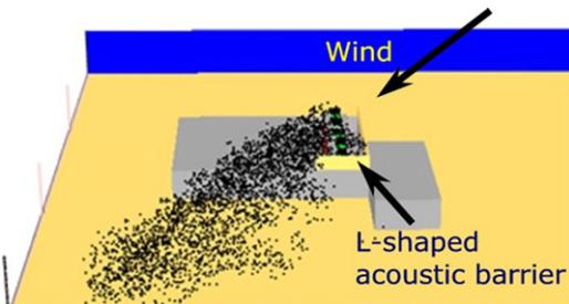
**Fig. 15.** An instantaneous snapshot, using SmokeView, of particles depicting the transport and dispersion of the cooling tower water-vapor plume. Note direction of wind and location of acoustic fence.
