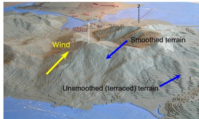
**Fig. 12.** Full view of scale model of Lantau Island near Hong Kong. Point 1 denotes the peak shown in Fig. 11. Because of poor representation of intermittent cycles of flow separation and reattachment, the CFD model was poor in simulating the flow at all locations between Points 1 and 2. Also note the smoothed and terraced portions of the terrain model in the study (from Derickson and Peterka, 2004).
