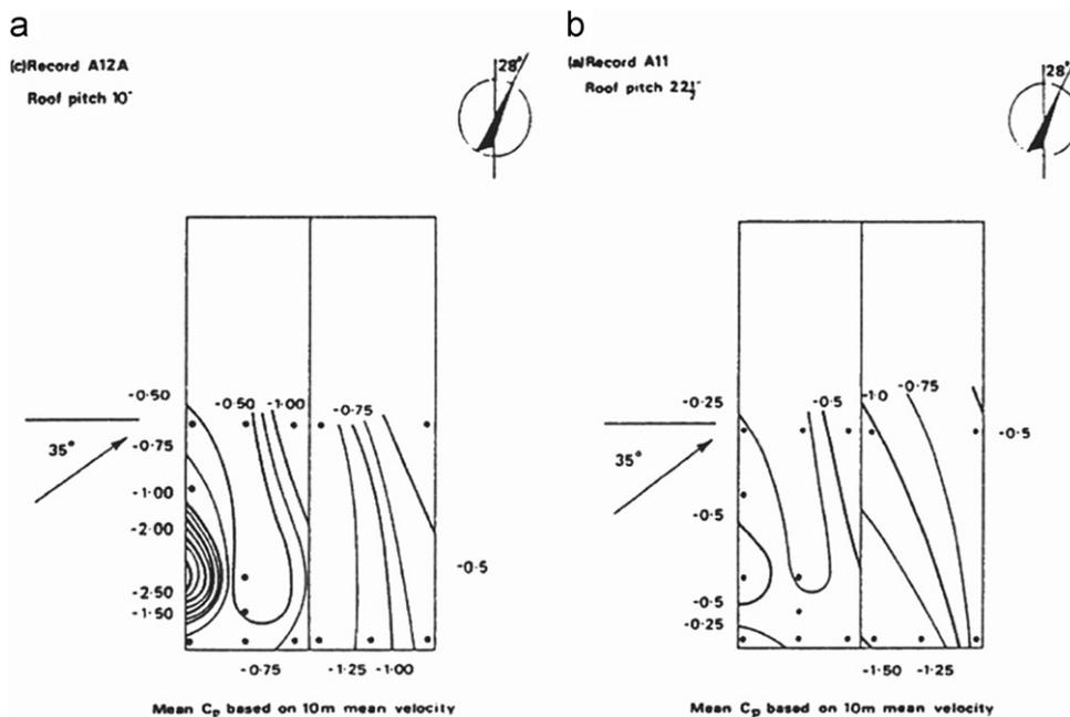
Fig. 2. Mean, full-scale pressure contours for cornering winds on two roof slopes (10° and 22.5°) of the Aylesbury House in Great Britain in the 1970s (after Eaton and Mayne, 1975).
