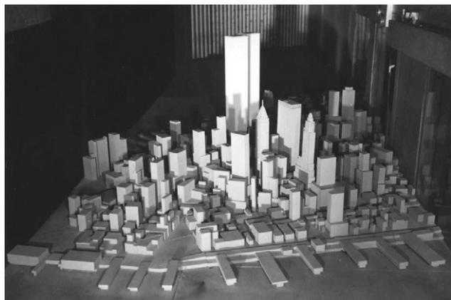
Fig. 1. Aeroelastic models of the World Trade Center, with surrounding Manhattan model, in one of the Colorado State University wind tunnels during the 1963/1964 studies.
