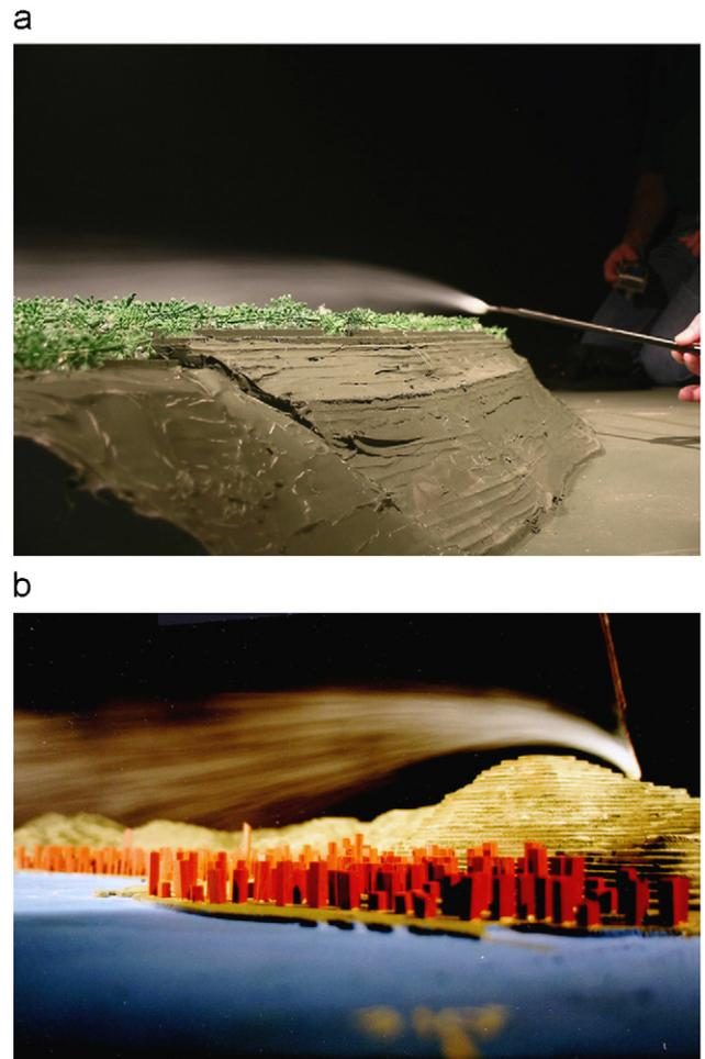
Fig. 13. Exploring flow separation on an escarpment model for a potential wind energy project (top) and over Victoria Peak on Hong Kong Island (bottom) for the wind structure at Central in the boundary-layer wind tunnel.
