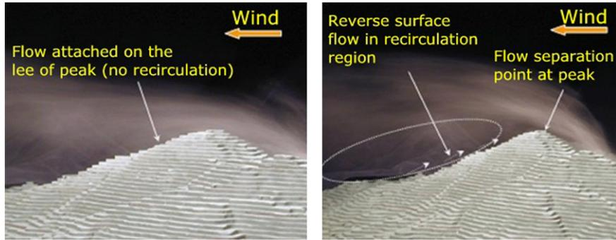
**Fig. 11.** Wind tunnel simulation showing intermittent flow separation and reattachment over a terrain peak on scale model of Lantau Island near Hong Kong. Modeling separation behavior with CFD can be erroneous and lead to misrepresentation of flow downwind of peak as shown by Derickson and Peterka (2004).
