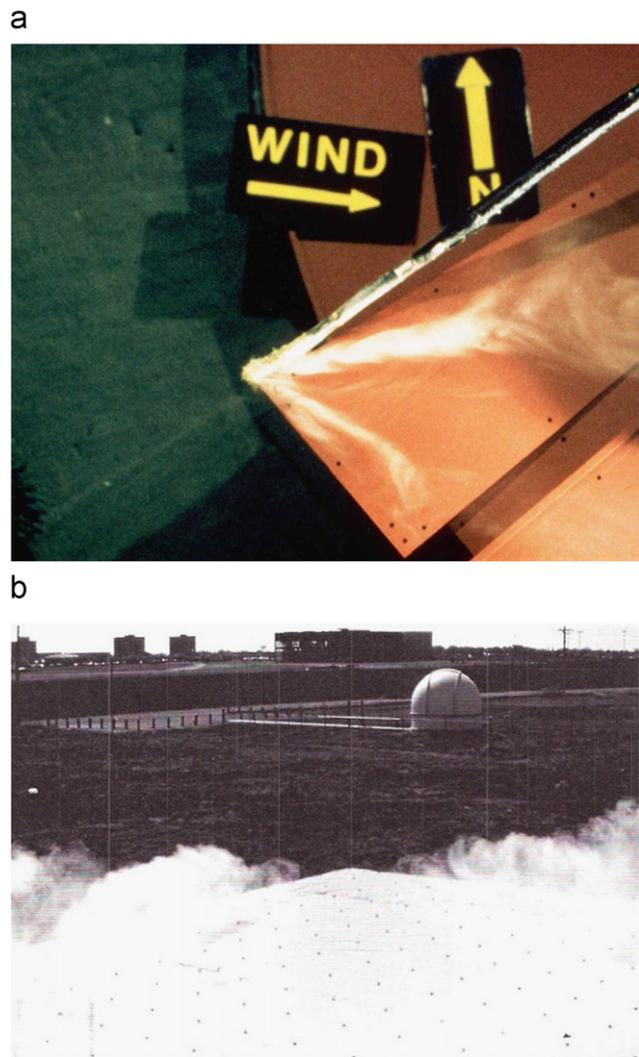
Fig. 5. Roof-corner vortices on a wind-tunnel model (top) and on the TTU Building (bottom).
