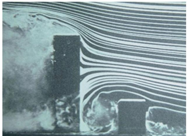
Fig. 17. Massively separated flow in the lee of the tall building (after Van Dyke, 1982).
